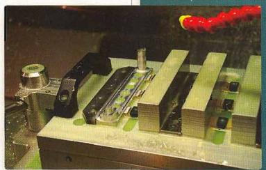
The X1Palletchanger lets operators load and reload a machine tool in less than 30 sec. In an unloading cycle, the operator unlocks the clamps, grasps the handles, and removes the platen. Loading is a matter of positioning the platen loaded with new work, placing it on the locators, and
